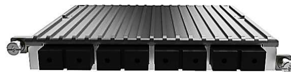
Модули 4 x 100/1000Base FO (MM/SM, SC/ST)
